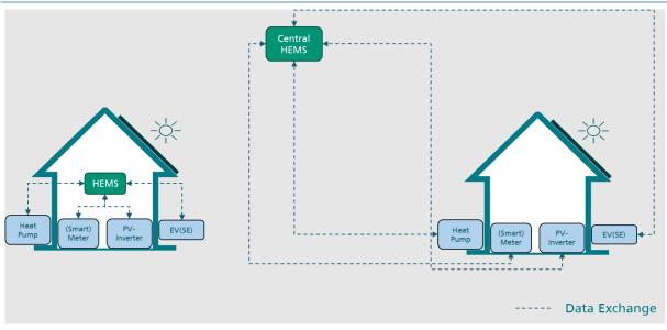
Figure 15: General approaches of HEMS architecture: decentral vs. central (simplified)
